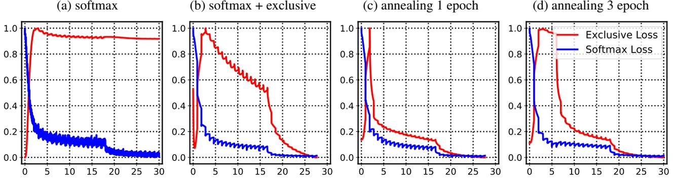
Figure 5. Exclusive loss under different annealing Strategies: (a): Softmax loss ( $\lambda = 0$ , without exclusive regularization). (b): Softmax loss + exclusive regularization, the exclusive term vibrates at the start of training. (c): Softmax + exclusive regularization with 1 epoch’s annealing, the exclusive term becomes more stable. (d): Softmax + exclusive regularization with 3 epoch’s annealing.
