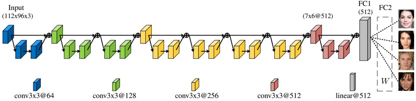
Figure 2. The ResNet20 architecture. ‘conv3x3@ $\mathcal{X}$ ’ represents a  $3 \times 3$  convolutional layer that outputs  $\mathcal{X}$  feature maps, and  $\oplus$  represents element-wise sum.  $W$  is a matrix that maps the facial representation to probabilities of input image belonging to identities.
