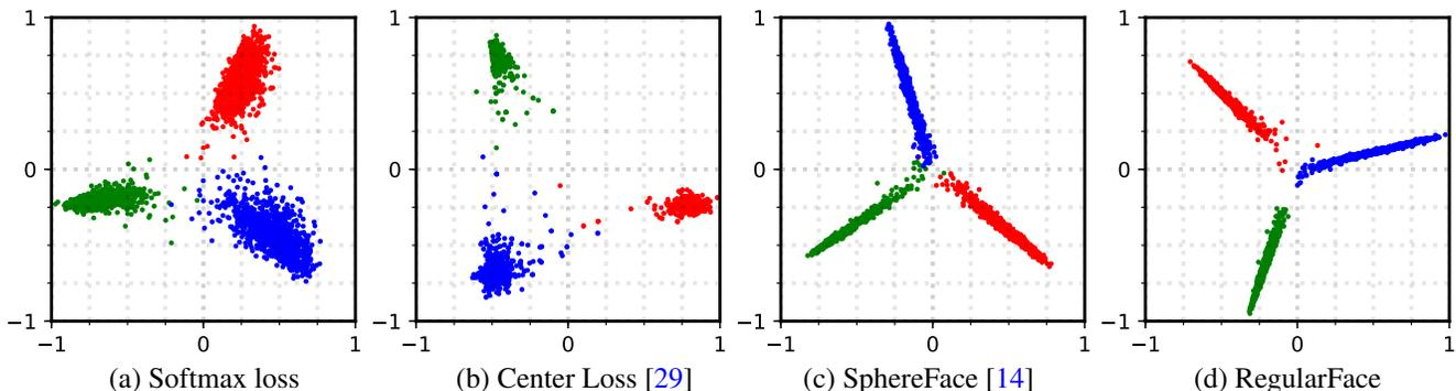
Figure 4. Representations of 3 digits MNIST classification. (a) Softmax loss learns separable representations; (b) Center loss[29] enhances intra-class compactness in the Euclidean space; (c) Sphreface[14] clamps intra-class representations in the sphere space; (d) Guided by the proposed exclusive regularization, inter-class representations present a mutual exclusive pattern, evidenced by large inter-class angles.
